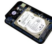
2. Insert the SATA drive into the SATA connector and secure the drive using the screws provided.
