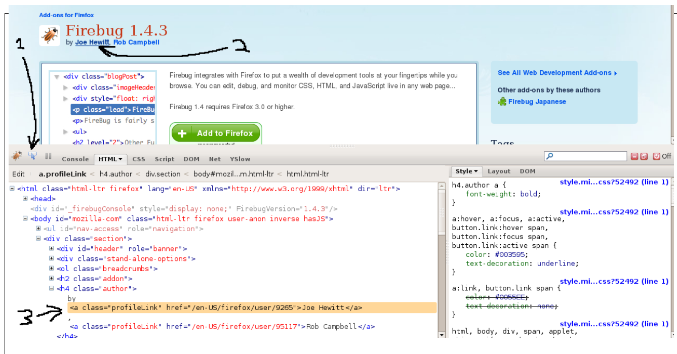
Figure 3-6. Firebug Inspector. 1) We click the inspector icon 2) We click on a page item ("Joe Hewitt") 3) Firebug shows the exact HTML element within the markup!
