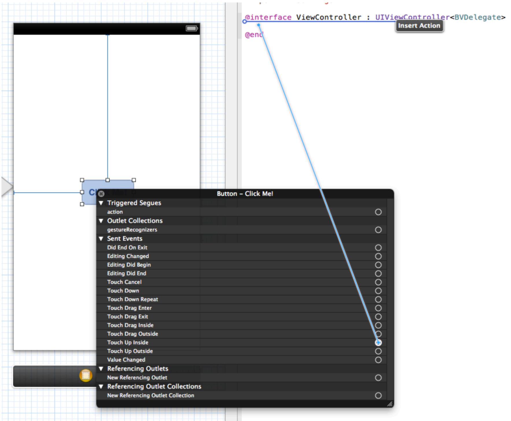
16. Set name to "clickedButton" and click "Connect." This will automatically insert code for the new action into **ViewController.h** and **ViewController.m**.
