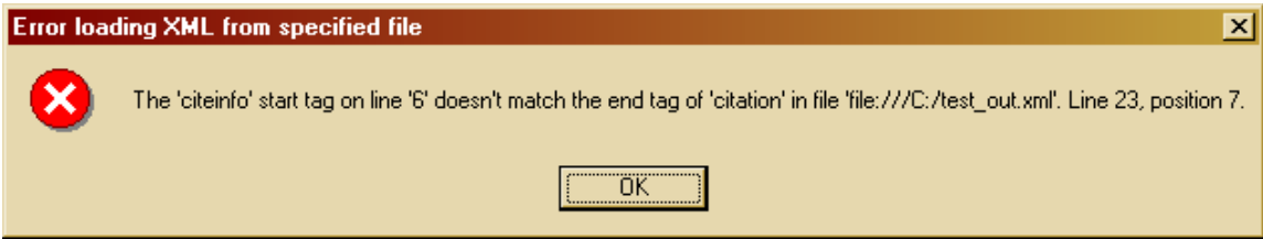
Figure 4.—Example error message when file being opened is not valid XML. The message displays what the program knows about where the XML error is.
